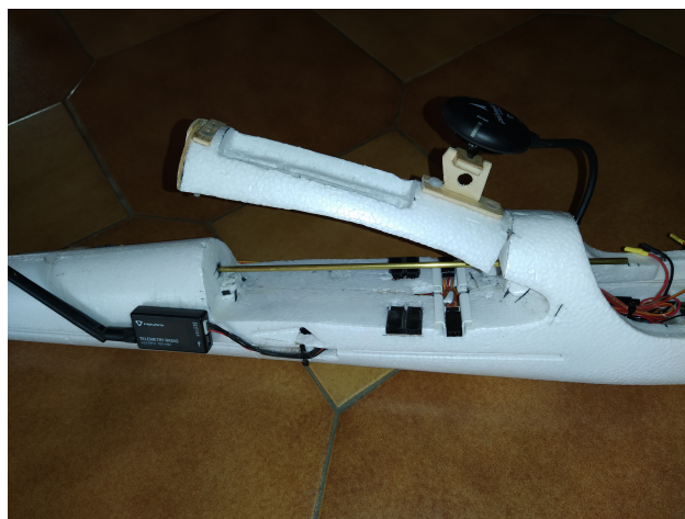
Fig. 2.7: Wing locking bar, which is a 4mm copper tube.
