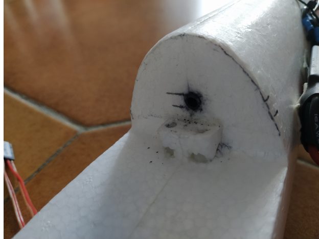
Fig. 2.6: 6mm carbon tube glued on the fuselage at the back of the wing. A similar tube is glued at the front.
