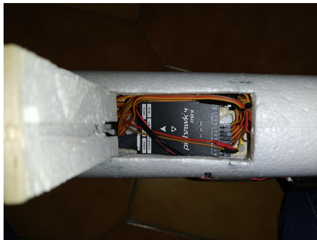
Fig. 3.1: The mini pixhawk board is mounted in the fuselage, below the wing.
